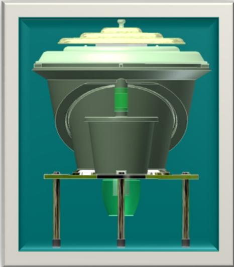
BSF bioconversion units (called *biopods*) are now being manufactured in a medium density polyethylene that lasts indefinitely. A nominal 2-foot diameter biopod (depicted on the left), weighing only 14 lbs (6.4 kg), can process over a metric ton of putrescent waste per year. A nominal 4-foot diameter biopod, weighing about 40 lbs (18 kg), can process well over five metric tons of putrescent waste per year.
